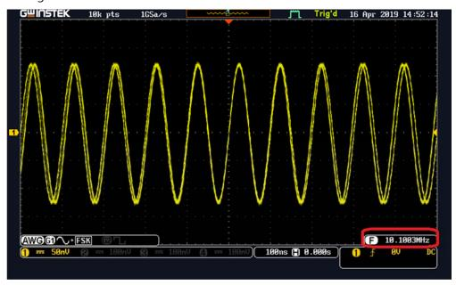
B. Set the center frequency of the Spectrum Analyzer by this frequency; set the start and stop frequencies to clearly observe the changing waveform of the FSK in the frequency domain.
