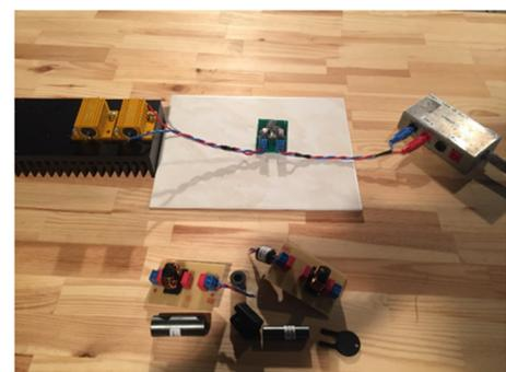
Fig. 23: Set-up for the measurement of the interference-field strength with and without external filters. The external filters should decouple the 20cm cable to ensure that only the emission of the circuit-board layout is measured
