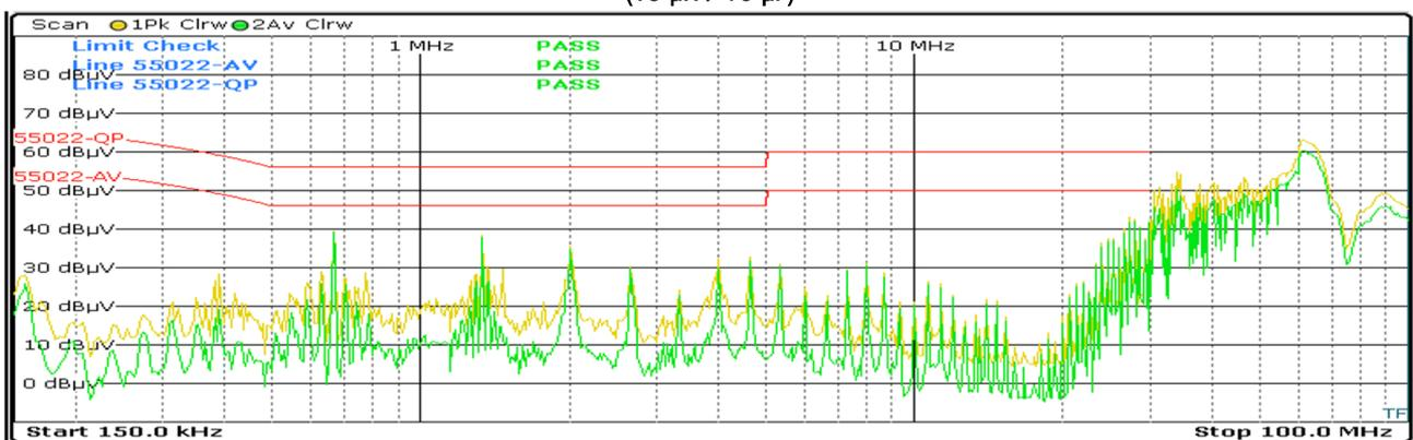
Figure 21: Measurement of the interference voltage of Design (1) at the **output** of the boost converter **with** LC filter (15  $\mu$ H / 10  $\mu$ F)
