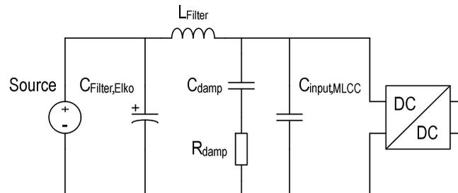
Figure 10: Measures for filter suppression: SMD resistor in series with a capacitor
