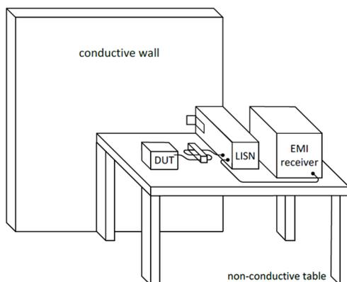
Figure 1: Test set-up for interfering voltage
