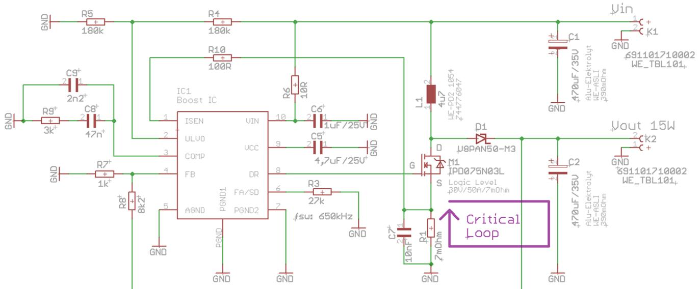
Figure 13: Circuit diagram of a critical design (Design 1) with  $U_{in} = 9\text{ V}$ ,  $U_{out} = 12\text{ V}$ ,  $I_{out} = 1.25\text{ A}$ ,  $f_{sw} = 650\text{ kHz}$
