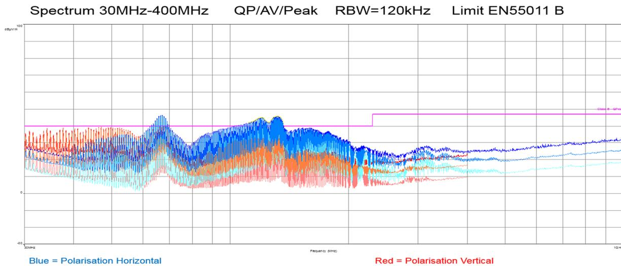
Fig. 24: Measurement of Design (1) **w**ith decoupling filters
