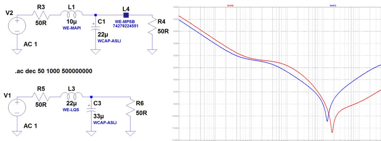
Figure 8: Simulated (LT Spice) suppression of a pure LC filter (22 $\mu\text{H}$  + 33 $\mu\text{F}$  blue) and a T filter (10 $\mu\text{H}$  + 22 $\mu\text{F}$  + MPSB 74279224551 red) in a 50 $\Omega$  system (1kHz - 500MHz).
