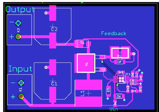
Figure 14: Circuit-board layout of the critical design (Design 1)
