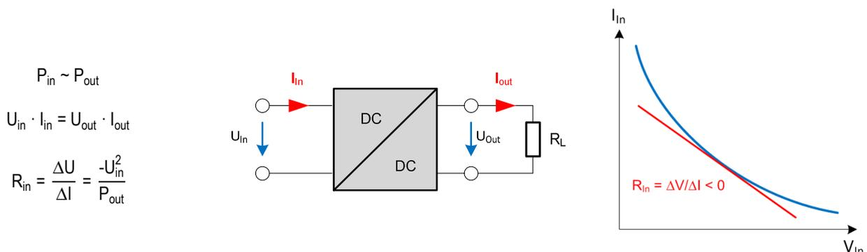
Fig. 9: Since the output remains constant even in the case of a drop in the input voltage, it is logical that the input current must rise. This results in a brief negative input resistance during this voltage transient.
