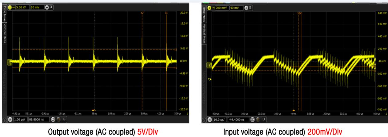
Figure 19: Measurement of the interferences in the time domain of Design (1) at the input and output of the boost converter **w/o** filter
