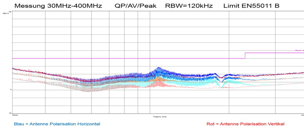
Figure 32: Measurement of design (2) **with** decoupling filters
