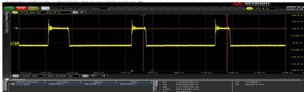
Figure 36: Measurement of the voltage over the Schottky diode
