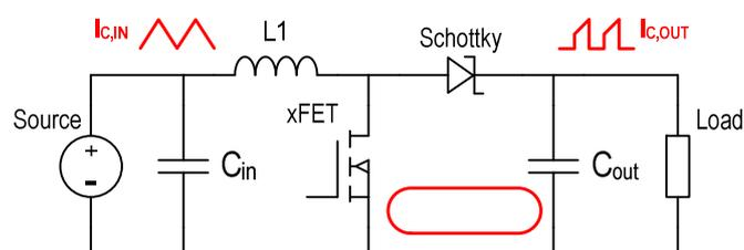
Figure 6: critical current loop **boost** converter
