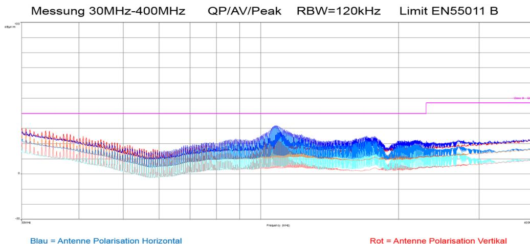
Figure 33: Measurement of design (2) **w/o** decoupling filters
