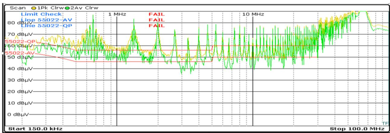
Figure 17: Measurement of the interference voltage of Design (1) at the **output** of the boost converter **w/o** filter
