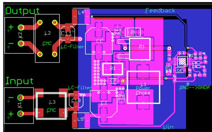
Fig. 16: Circuit-board layout of the good design (Design 2)
