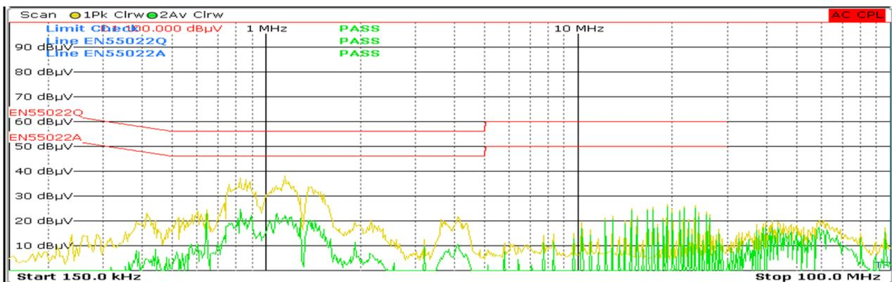
Figure 30: Measurement of the interference voltage of Design (2) at the **input** of the boost converter with filter (15 µH / 10 µF / Stroko 5 µH)
