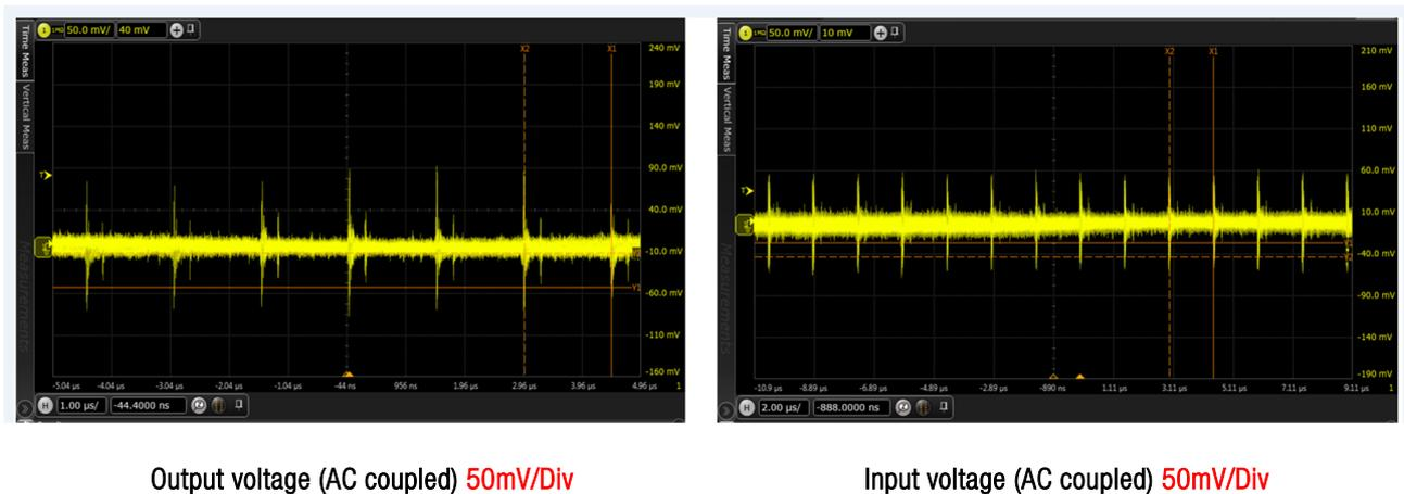
Figure 20: Measurement of the interferences in the time domain of Design (1) at the input and output of the boost converter **with** LC filter (15  $\mu$ H / 10  $\mu$ F)
