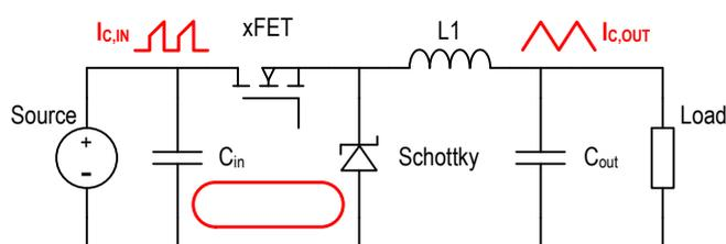
Figure 5: critical current loop **buck** converter
