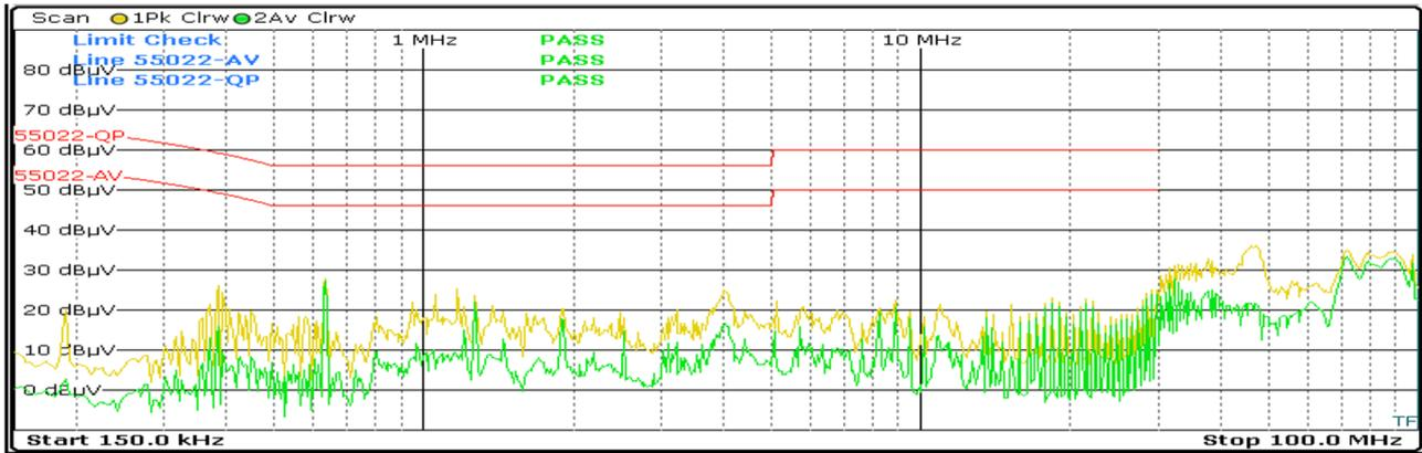
Figure 29: Measurement of the interference voltage of Design (2) at the **output** of the boost converter **with filter** (15 µH / 10µF / Stroko 5 mH)
