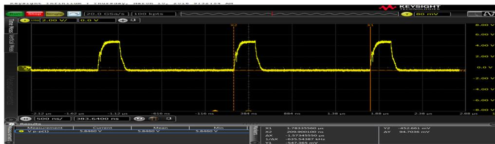
Figure 34: Measurement of the gate-source voltage at the MOSFET
