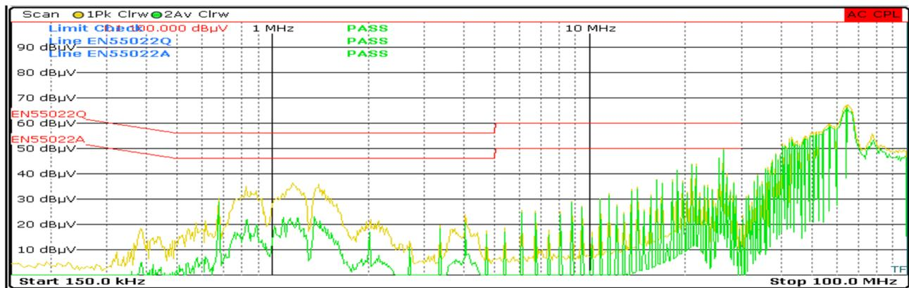
Figure 22: Measurement of the interference voltage of Design (1) at the **input** of the boost converter **with** LC filter (15 µH / 10 µF)
