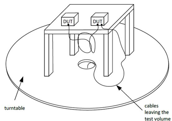
Figure 2: Test set-up for interference-field strength with turntable
