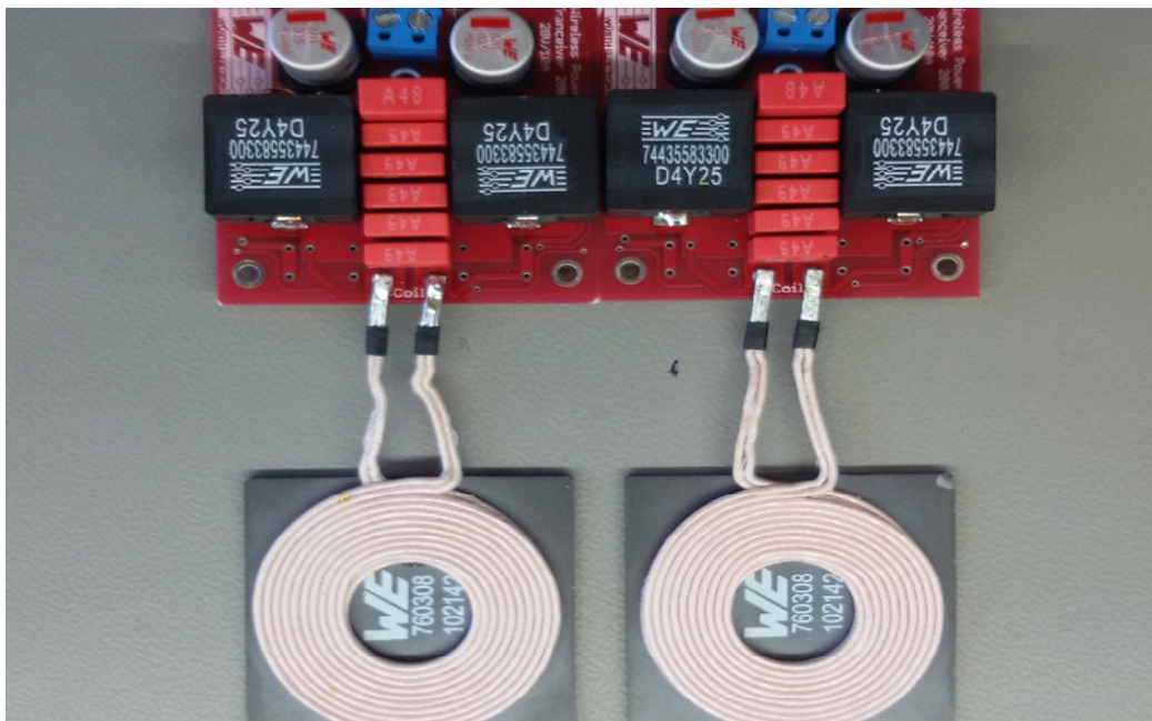
Figure 7: Measured circuit ( V_{in} = 20 \text{ VDC} ; P_{out} = 100 \text{ W} ) for a 6.5 mm air gap
