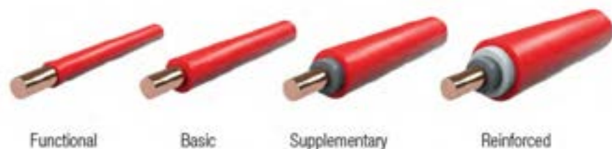
Figure 5. A distinction is made between functional, basic, supplementary and reinforced wire insulation
